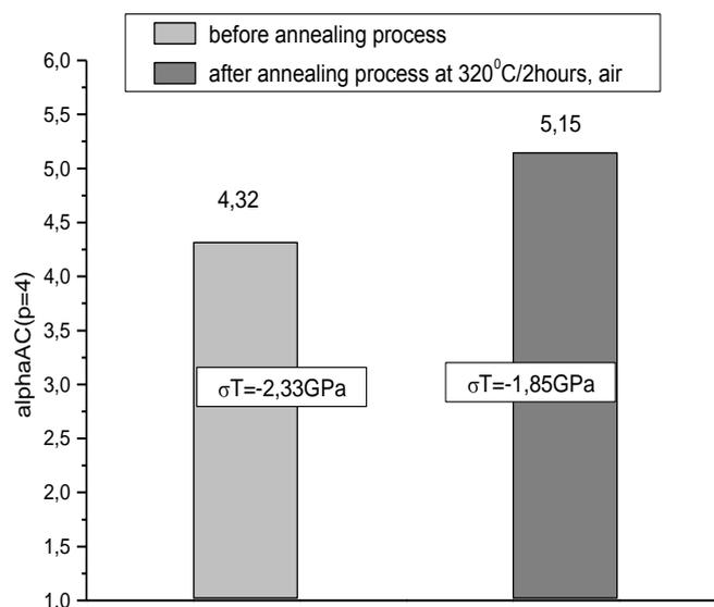
Figure presents the result of testing the thermal stability of TiN thin film coated on iron substrate in the shape of thin ribbon, annealed at 320°C by 2 hours in the air atmosphere. The coefficient of the thermal expansion (CTE) is in relation with the volume of stress obtained from XRD.
